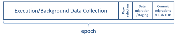
Fig. 1. A sample epoch showing the large computational period and the smaller migration-related periods.
